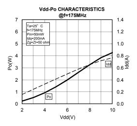
RoHS Compliant, Silicon MOSFET Power Transistor 175MHz,520MHz,2W
