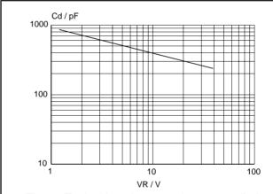
Fig.5. Typical junction capacitance per diode;  $C_d = f(V_R)$ ; f = 1 MHz;  $T_j = 25$ °C to 125°C.
