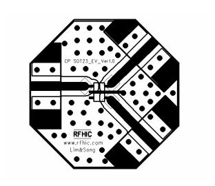
PCB material (FR4), PCB thickness (0.8t), Via hole ( $\Phi$ 0.7)
