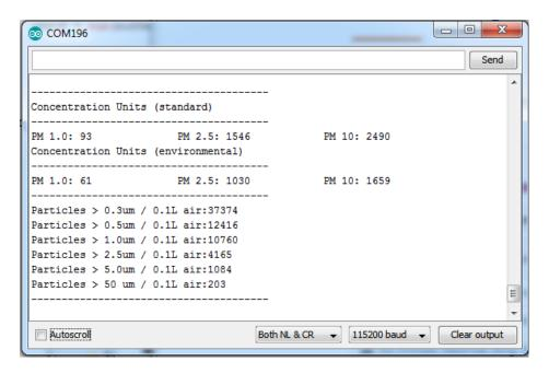
Note that the numbers are very precise looking but we don't believe that they're going to be perfectly accurate, calibration may be necessary!
