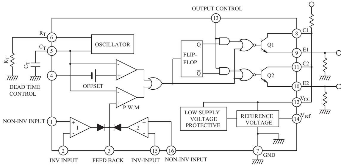
(Note) PIN ⑬ BECOMES SINGLE MODE AT "L" AND PUSH-PULL MODE AT "H"
