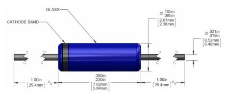
Lead Material: copper clad steel
