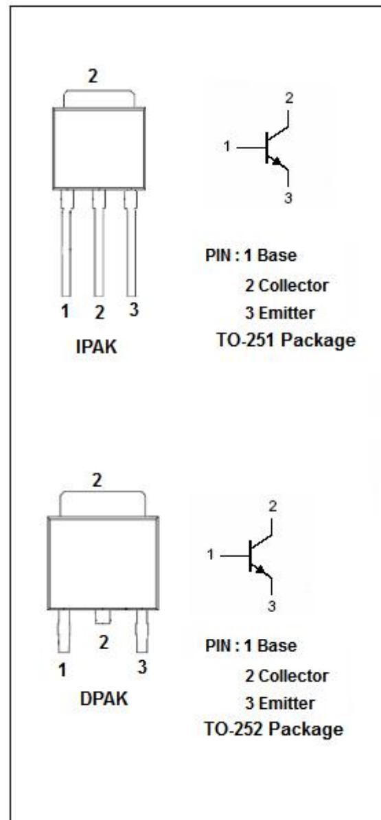
**isc Silicon NPN Power Transistor****2SC4027****ELECTRICAL CHARACTERISTICS****T<sub>c</sub>=25°C unless otherwise specified**
