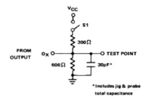
This is the A.C. Test Load which Harris Semiconductor uses in its automatic test equipment, and it is recommended that users of Harris bipolar devices use the same or an equivalent load in performing A.C. testing.
