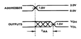
NOTE: As is common to all memory devices, output levels can be undefined during the address access period (TAA); however, the outputs are guaranteed to reach stable levels by TAA. It is not recommended that outputs from this class of devices be used to drive edge triggered inputs on subsequent devices (counters, filip-fiops, etc.) without proper intermediate synchronization.
