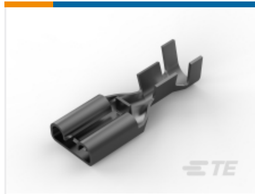
TE Part # 63854-2 250 PL MKIII REC. 18-14AWG TPBR
