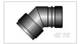
Connector Backshell Product Style: Unscreened Connector Backshell Product Type: Backshell Primary Product Material: Aluminum Alloy Body Orientation: 45° Connector Interface Specification: MIL-C-38999 Series III & IV
