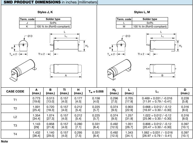
Use appropriate adhesive between capacitor body and the board for improved mechanical strength
