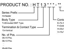
Modification Code None-Standard Product P2=With 2 Post - Contact Area Plating E=Tin Plating With RoHS COMPLIANCE F=Gold Flash With RoHS COMPLIANCE H=30u" Gold With RoHS COMPLIANCE
