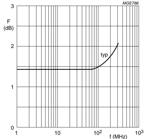
$V_{DS} = 15$  V;  $V_{GS} = 0$ ;  $R_G = 1$  k $\Omega$ ;  $T_{amb} = 25$  °C.
