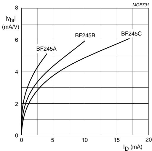
$V_{DS} = 15$  V;  $f = 1$  kHz;  $T_{amb} = 25$  °C.
