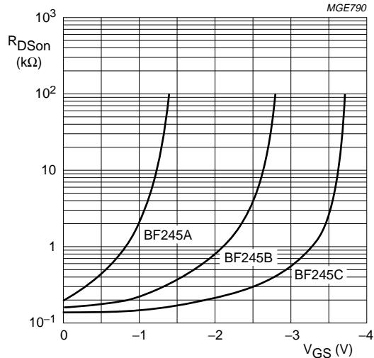
$V_{DS} = 0$ ;  $f = 1$  kHz;  $T_{amb} = 25$  °C.
