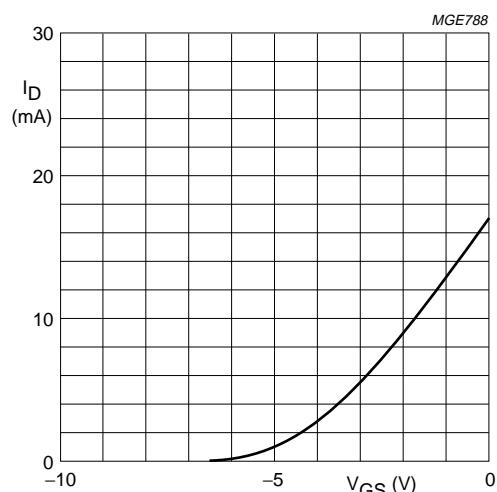
$V_{DS} = 15\text{ V}; T_j = 25\text{ }^\circ\text{C}$ .Fig.7 Transfer characteristics for BF245C;
