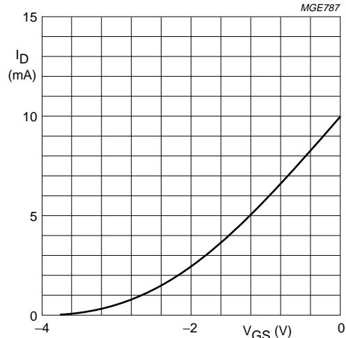
$V_{DS} = 15\text{ V}; T_j = 25\text{ }^\circ\text{C}$ .Fig.5 Transfer characteristics for BF245B;
