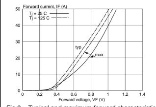
Fig.3. Typical and maximum forward characteristic  $I_F = f(V_F)$ ; parameter  $T_i$
