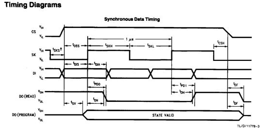
$t_{SKS}$  is not needed if DI =  $V_{IL}$  when CS is going active (HIGH).
