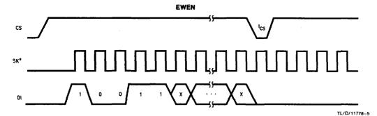
\*The NM93C56LZ and NM93C66LZ require a minimum of 11 clock cycles. The NM93C06LZ and NM93C46LZ require a minimum of 9 clock cycles.
