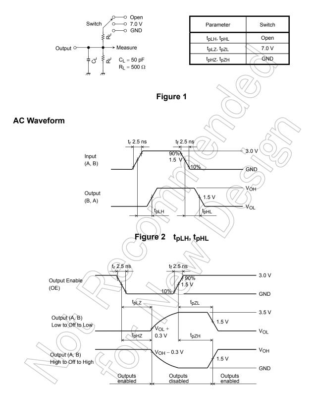
Figure 3  $t_{pLZ}$ ,  $t_{pHZ}$ ,  $t_{pZL}$ ,  $t_{pZH}$
