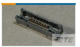
TE Part #5767171-1 MICTOR RECEPT ASSY, 38 POS. TA
