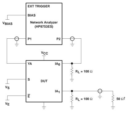
$<sup>\</sup>dagger$  A 50-Ω termination resistor is needed for the network analyzer.
