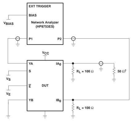
$\dagger$  A 50- $\!\Omega$  termination resistor is needed for the network analyzer.
