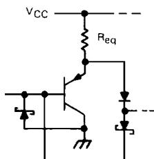
Count/Load, Clear:  $R_{req} = 2.3 \text{ k}\Omega \text{ NOM}$
