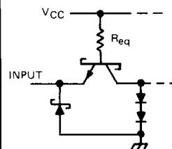
Clock 1  $R_{req} = 1.2 \text{ k}\Omega \text{ NOM}$
