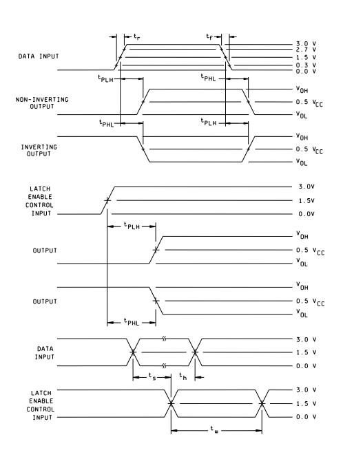
FIGURE 5. Switching waveforms and test circuit.
