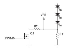
$$MOSFET 'off' \\ I_{LED(MIN)} = \frac{V_{FB}}{R_{LED}}$$
