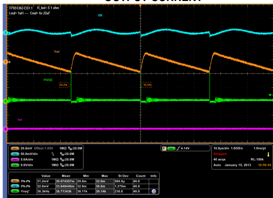
Figure 17. f = 400\text{kHz} , V_{\text{IN}} = 20\text{V} , I_{\text{OUT}} = 0.1\text{A}
