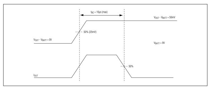
Figure 1. Back-Charge Turn-Off Time
