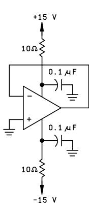
FIGURE 2. Radiation exposure circuit.
