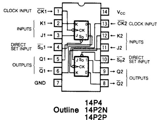
just previously input at J and K appear at outputs Q and  $\overline{Q}$  in accordance with the function table given. When  $\overline{S_D}$  is low, Q and  $\overline{Q}$  will become high and low respectively, irrespective of other inputs. When used as a J-K flip flop,  $\overline{S_D}$  should be maintained at high-level.
