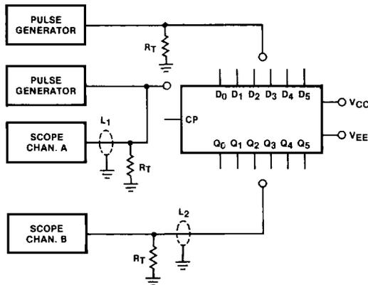
$L_1$  and  $L_2$  = equal length  $50 \Omega$  impedance lines
