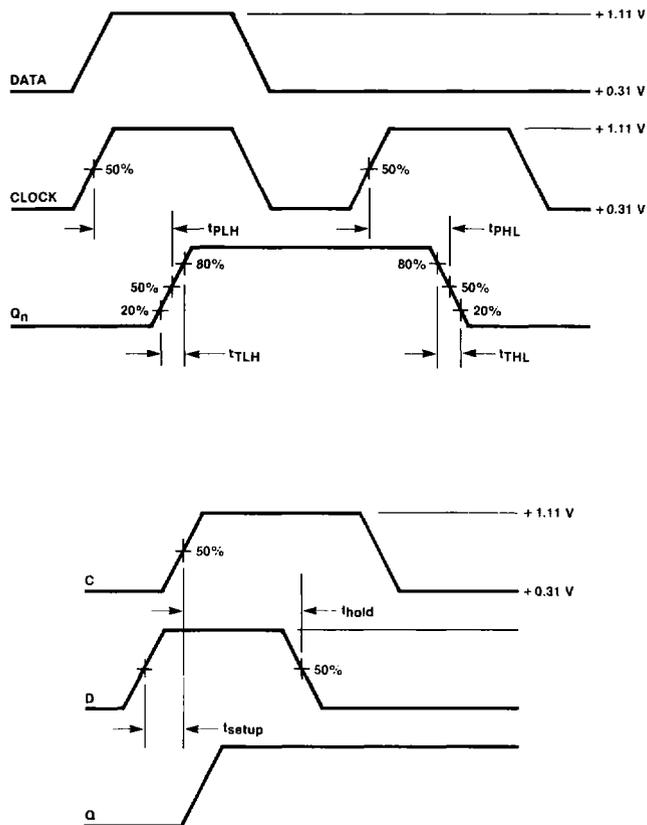
$t_{setup}$  is the minimum time before the transition of the clock pulse (C) that information must be present at the data input (D).
