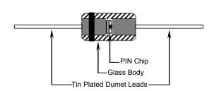
MACOMs silicon PIN diode chips are also available in a wide variety of alternative package styles besides glass. For case style options, availability and electrical specifications, please refer to the "Packaged PIN Diode Datasheet" located on the MACOM website.
