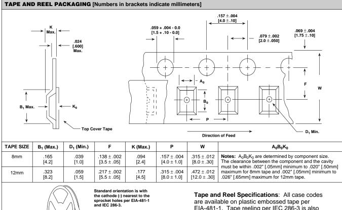
are available on plastic embossed tape per EIA-481-1. Tape reeling per IEC 286-3 is also available. Standard reel diameter is 13" [330mm]. 7" [178mm] reels are available.
