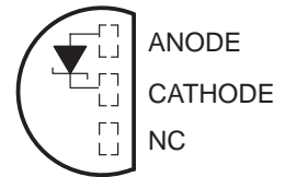
1.2 V . . . LP (TO-92/TO-226) PACKAGE (TOP VIEW)
