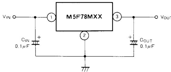
**ELECTRIC CHARACTERISTICS****M5F78M05** ( $V_{IN} = 10V$ ,  $I_0 = 350mA$ ,  $0^\circ\text{C} \leq T_J \leq 125^\circ\text{C}$ )
