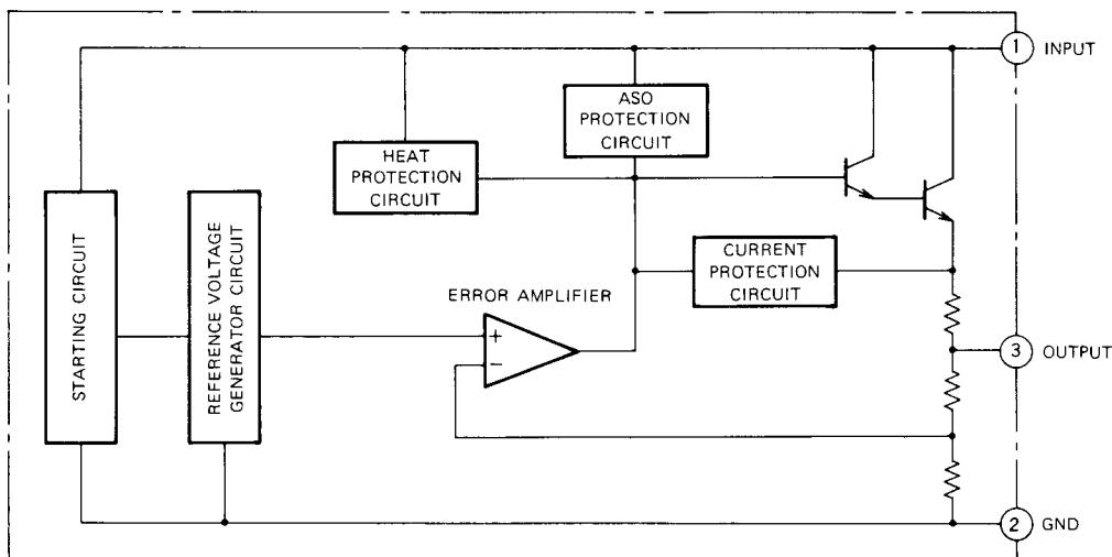
**FIXED POSITIVE OUTPUT 3-Terminal Regulator Series****ABSOLUTE MAXIMUM RATINGS** ( $T_a = 25^\circ\text{C}$ , unless otherwise noted)
