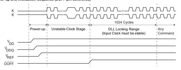
Power-up and Initilization Sequence (DOFF pin fixed HIGH, clock controlled)
