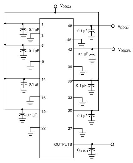
Note: All capacitors should be placed as close to each pin as possible.
