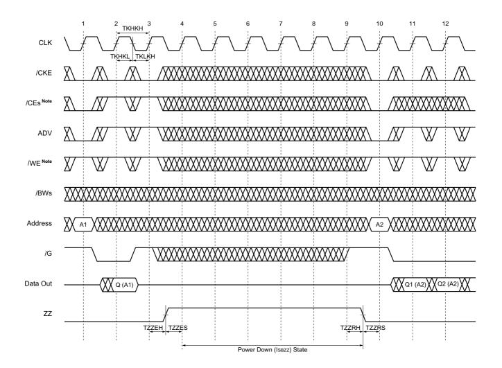
**Note** /WE or /CEs must be held HIGH at CLK rising edge (clock edge No.3 in this figure) prior to power down state entry.
