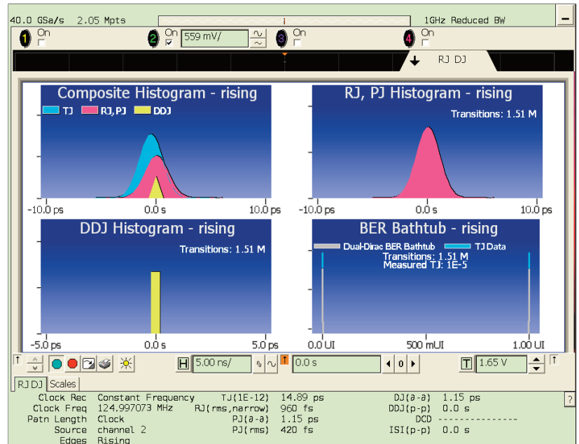
Figure 1: Jitter Analysis of a QT82LD-125MHZ
