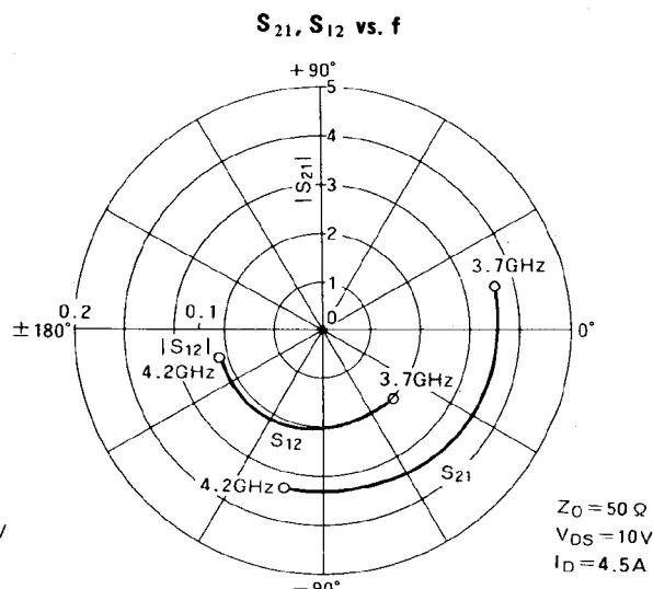
**S PARAMETERS** ( $T_a = 25^\circ\text{C}$ ,  $V_{DS} = 10V$ ,  $I_{DS} = 4.5A$ )
