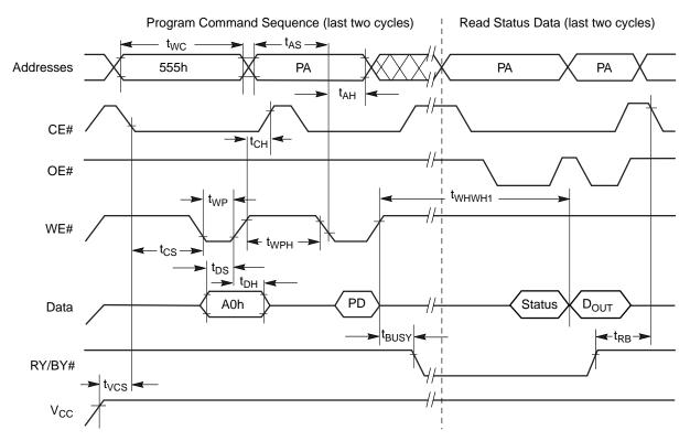
**Note:**  $PA = program \ address, PD = program \ data, D_{OUT}$  is the true data at the program address.
