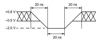
Figure 6. Maximum Negative Overshoot Waveform
