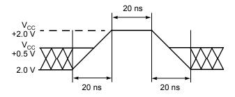
Figure 7. Maximum Positive Overshoot Waveform
