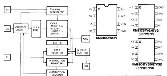
\*Note: When the ORG pin is connected to V<sub>CC</sub>, X16 organization is selected. And when it is connected to ground, X8 organization is selected. If it is unconnected, then an internal pull-up device will select the X16 organization.
