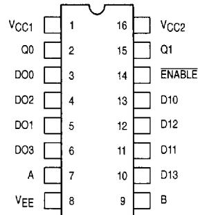
Pin assignment is for Dual-in-Line Package.
