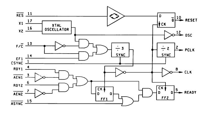
FIGURE 2. Block diagram.
