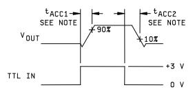
NOTE:  $\mathtt{t}_{ACC}$  IS DEFINED AS THE LONGEST OF  $\mathtt{t}_{ACC1}$  AND  $\mathtt{t}_{ACC2}.$  ACCESS TIME
