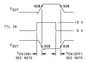
NOTE:  $t_{\mbox{EN (ON/OFF)}}$  IS DEFINED AS THE LONGEST OF +5 V AND-5 V INPUT CASE. ENABLE DELAY
