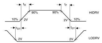
Figure 2. Output Drive Timing Diagram
