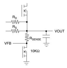
Figure 6. Using VADJ to Generate VTT
