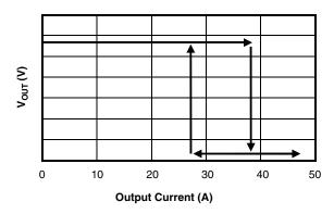
Figure 3. FAN5056 Short Circuit Characteristic
