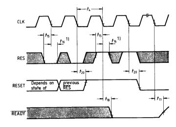
$<sup>^{\</sup>scriptsize 1)}$  This is an asynchronous input. The setup and hold times shown are required to guarantee the response shown.
