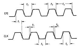
The EFI input low and high times as shown are required to guarantee the CLK low and high times shown.
