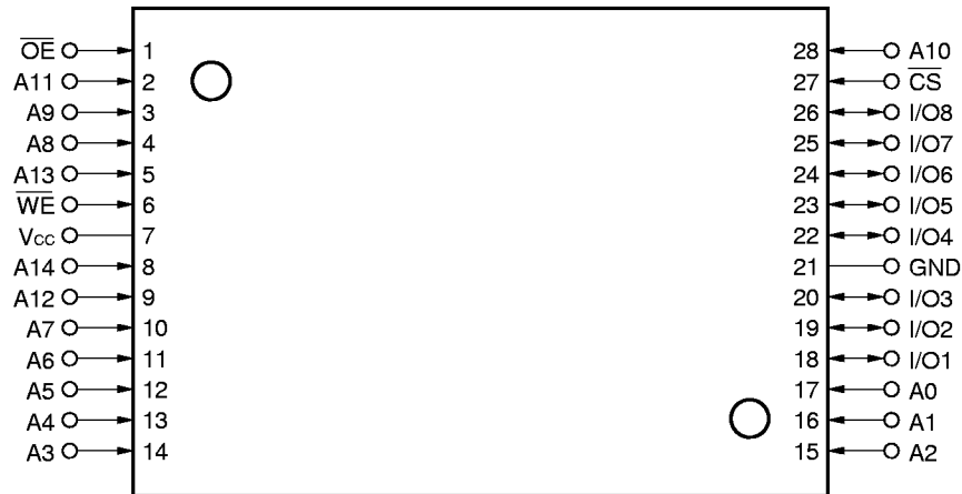
28-pin plastic TSOP (I) (8 × 13.4mm) (Normal bent)
