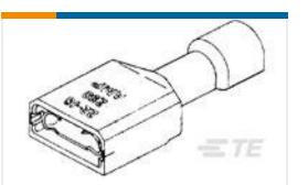
TE Part #3-520408-2 ULTRA-FAST 250 ASY REC 16-14 AWG TPBR
