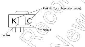
Note 3: A line to the right of a Lot No. identifies the indication of product Labels. Without a line: [[Pb]]/INCLUDES > MCV With a line? [[G]]/RoHS COMPATIBLE or [[G]]/RoHS [[Pb]]
