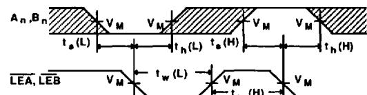
Waveform 2. Data Setup And Hold Times And LEA, LEB Pulse Widths
