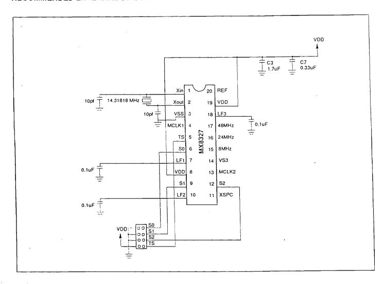
Note: S0, S1, S2 internal pull-up TS internal pull-down
