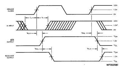
Note: Bus to Receiver output delay is measured by clocking data into the driver register and measuring the BUS to R combinatorial delay.
