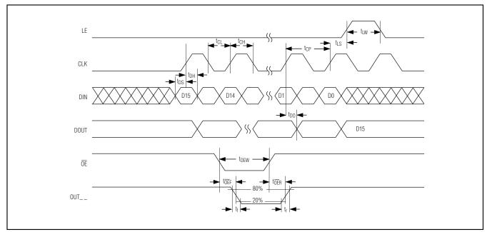
Figure 3. 4-Wire Serial-Interface Timing Diagram
