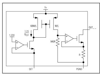
Figure 1c. OUT\_ \_ Driver Internal Diagram
