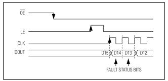
Figure 5. Fault Timing
