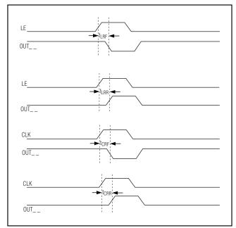
Figure 4. LE and CLK to OUT\_ \_ Timing
