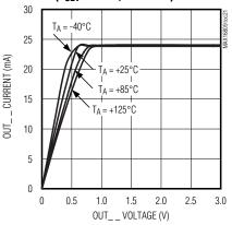
$\begin{array}{l} \textbf{OUT}\_ \ \textbf{CURRENT vs. } \textbf{OUT}\_ \ \textbf{VOLTAGE} \\ \textbf{(R}_{SET} = 720\Omega, \ \textbf{V+} = 5.0\textbf{V}) \end{array}$
