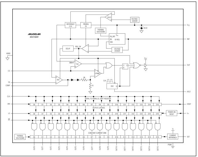
Figure 1a. Internal Block Diagram (MAX16809)
