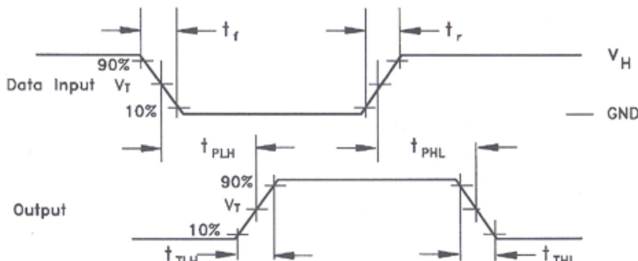
Input and Output threshold voltage, V<sub>T</sub>=50% V<sub>CC</sub> for HC; 1.3V for HCT
